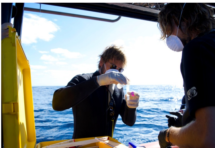
Figure 2: Preparation of collected samples on board the research vessel. Cross contamination between samples and from involved staff posed one of the biggest challenges.
